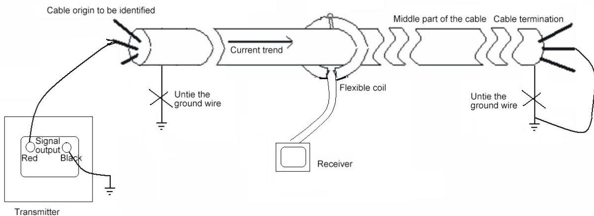
(1) Connect the output coupling pliers respectively according to the color, use AC240V for the launching host or install four pieces of AA alkaline battery, and connect the output calipers to the cable to be identified according to the direction marked by the pliers.
