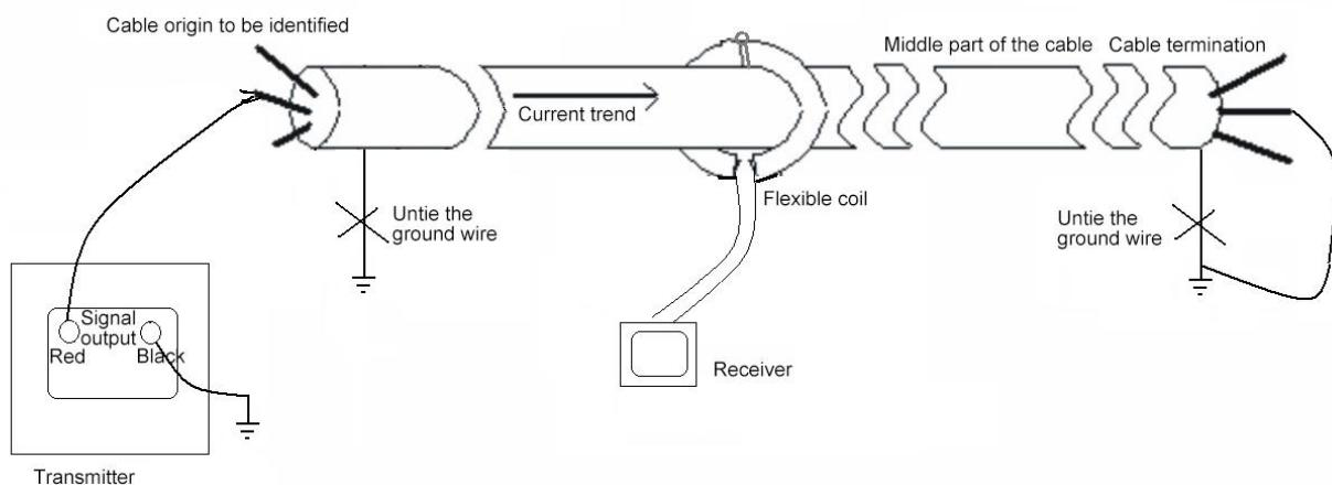
The difference with the live cable identification is: do not use the transmitter calipers, untie the start and end of the cable to be identified, untie the armor wires on both sides, use the dedicated direct connection output wire, the red wire is connected to the cable core wire, and the black wire is connected to the earth, the cable core wire terminal is connected to the earth. Refer to 1 for other operations.
